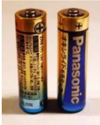
A pair of AA cells. The + sign indicates the terminal with the highest electric potential.
