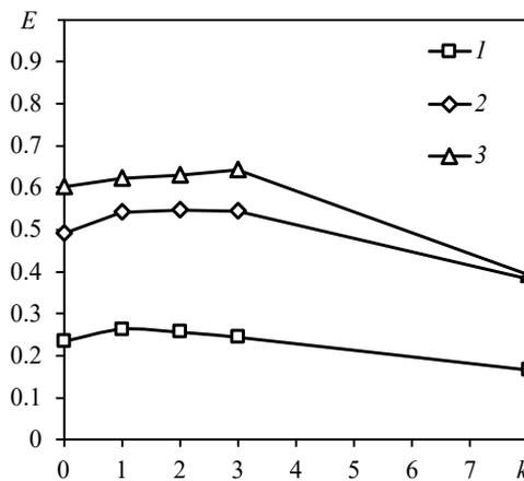
**Fig. 4.** Separation efficiency versus number of sloped blades  $k$  at different gas input velocity  $W$ , m/s: (1) 3; (2) 7; (3) 10
