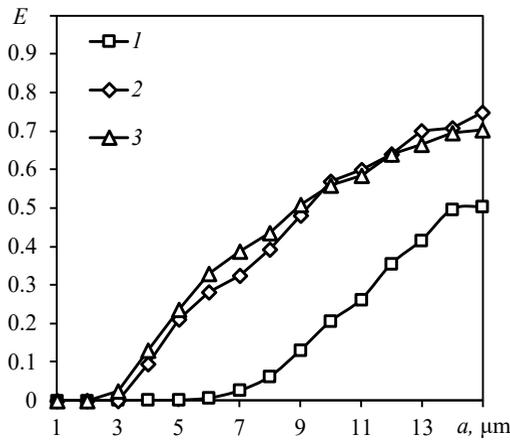
**Fig. 3.** Separation efficiency vs. particle size at different inlet gas velocity  $W$ , m/s: (1) 3; (2) 7; (3) 10 ( $k = 8$ )
