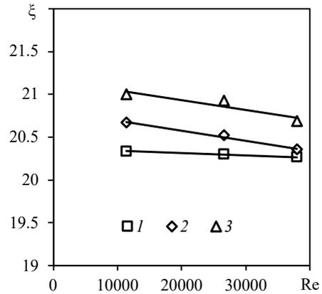
**Fig. 6.** Hydraulic resistance coefficient vs. Reynolds number for different numbers of sloped blades  $k$ , pcs.: (1) 0; (2) 1; (3) 8
