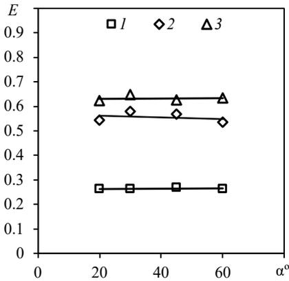
**Fig. 5.** Separation efficiency vs. angle of slope of the blades at different inlet gas velocity  $W$ , m/s: (1) 3; (2) 7; (3) 10
