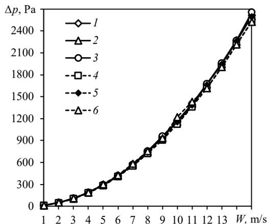
**Fig. 2.** Pressure drop vs. inlet gas velocity for various turbulence models: 1 – Spalart–Allmaras; 2 –  $k-\epsilon$  Standard; 3 –  $k-\omega$  Standard; 4 –  $k-kl-\omega$ ; 5 –  $k-\omega$  SST; 6 – RSM
