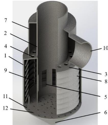
**Fig. 1.** Static centrifugal multi-vortex separator: (1) external pipe No 1; (2) internal pipe; (3) baffle plate; (4), and (12) holes; (5) apertures; (6) conical hopper; (7) external pipe No 2; (8) sloped blades; (9) studs; (10) outlet; (11) bottom.
