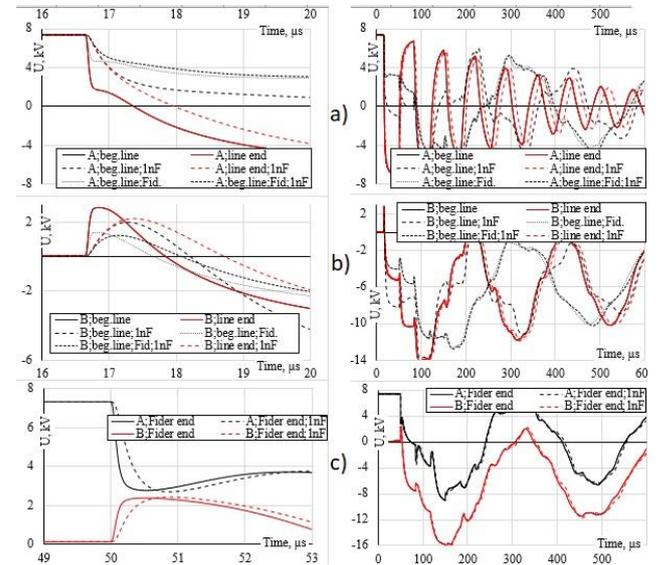
Fig. 4. Time dependences of voltage TS in a three-phase line.
