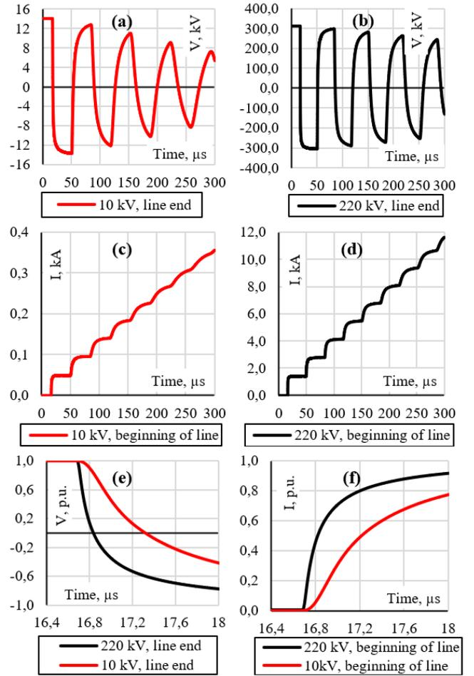
Fig. 3. Time dependences of current and voltage TS in a simple single-phase line for 10 and 220 kV line.
