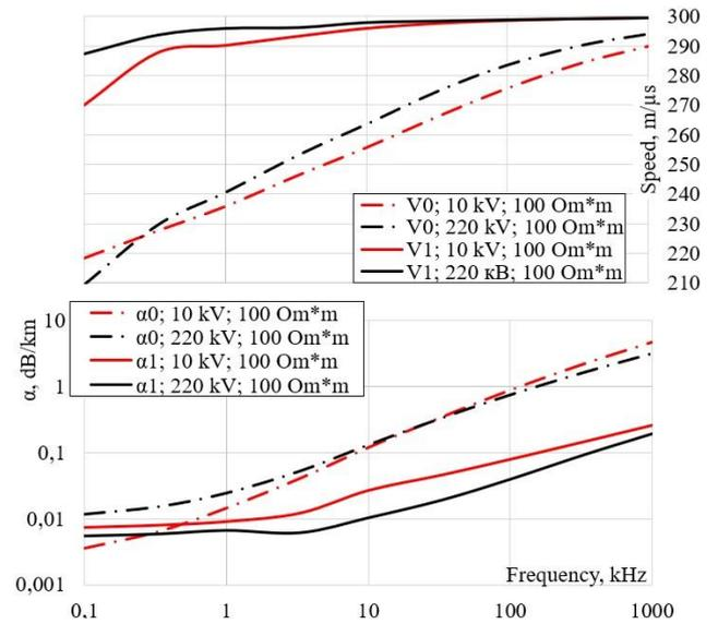
Fig. 1. Frequency dependences of modal phase speed and decay constant.
