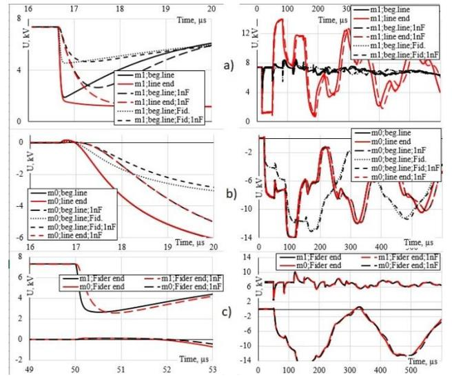
Fig. 5. Time dependencies of modal TS voltage for three-phase line.
