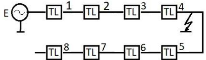
Fig. 2. Schematic of a line consisting of 8 identical sections of 1.25 km length.
