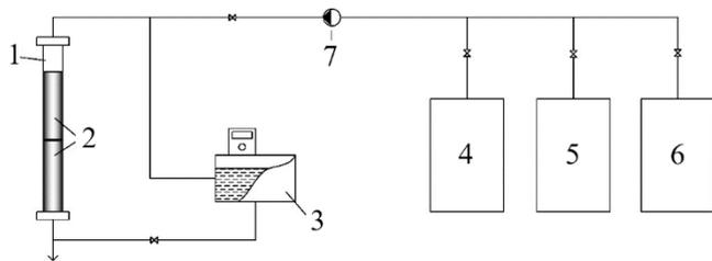
Fig. 1. Laboratory installation of a mixed-bed filter. 1 - magnetic water treatment unit; 2 - clarifier; 3 - clarified water tank; 4, 5 1 - ion exchange column; 2- monodisperse copolymer of styrene with divinylbenzene brands TOKEM-140 and TOKEM-840 in a ratio of 60/40; 3- liquid thermostat LOIP LT-108a; 4 - HCl block; 5 - NaOH block; 6 - distilled water; 7 - water pump.
