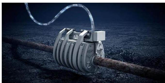
Figure 3. Robot for underwater repair. [3]
