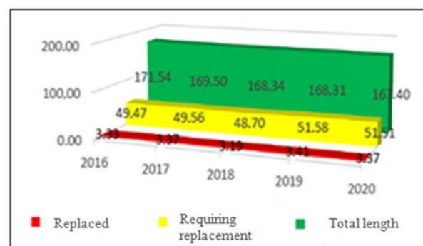
**Fig. 1.** The ratio of the total length of heating networks with the length of networks in need of replacement and replaced in the Russian Federation in 2016-2020, thousand km.
