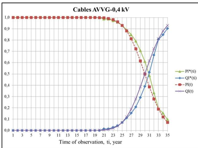
Fig 8. Graphical dependences of change in time of  $P_1^*(t_i)$ ,  $Q_1^*(t_i)$ ,  $P_1(t)$  and  $Q_1(t)$  for cables AVVG-0,4 kV
