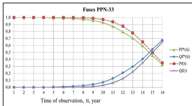
Fig 5. Graphical dependences of change in time  $P_F^*(t_i)$ ,  $Q_F^*(t_i)$ ,  $P_F(t)$  and  $Q_F(t)$  for PPN-33 fuses
