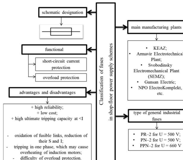
Fig 1. Classification of fuses in shop-floor power supply schemes
