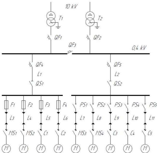
Fig 4. Schematic diagram of the workshop network section
