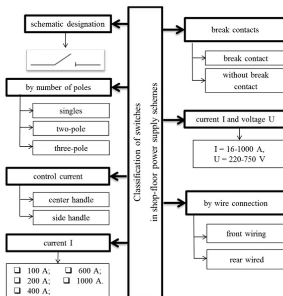
Fig 2. Classification of switches in shop-floor power supply schemes
