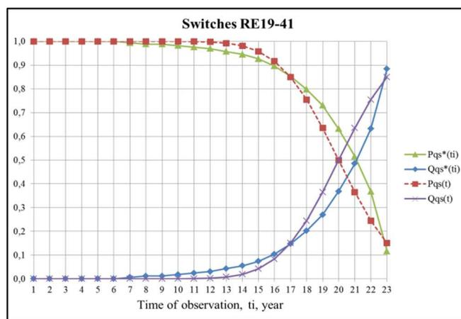
Fig 6. Graphical dependences of change in time of  $P_{qs}^*(t_i)$ ,  $Q_{qs}^*(t_i)$ ,  $P_{qs}(t)$  and  $Q_{qs}(t)$  for switches RE19-41
