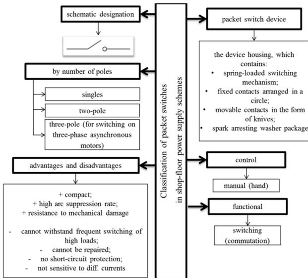
Fig 3. Classification of packet switches in shop-floor power supply schemes
