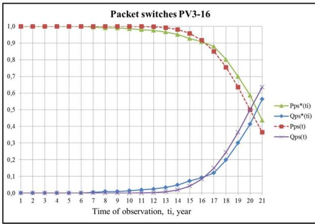
Fig 7. Graphical dependences of change in time of  $P_{ps}^*(t_i)$ ,  $Q_{ps}^*(t_i)$ ,  $P_{ps}(t)$  and  $Q_{ps}(t)$  for packet switches PV3-16
