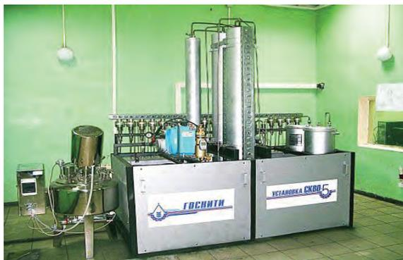
Figure 2 – Installation for the implementation of the SCWO
