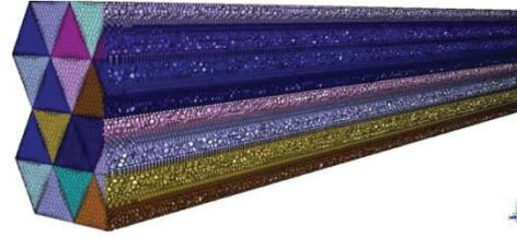
**FIGURE 12.** Three-dimensional model of heat transfer plates with crinkle and straight plates
