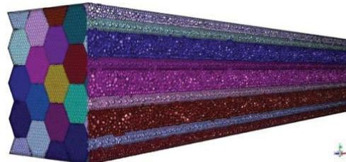
**FIGURE 10.** Three-dimensional model of heat exchange plates with "honeycomb" channels
