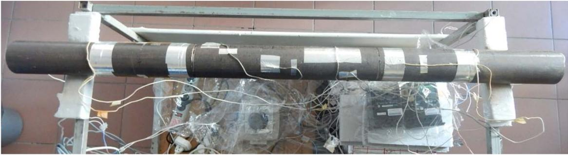
Fig. 2. Experimental apparatus. Guarded hot pipe.
