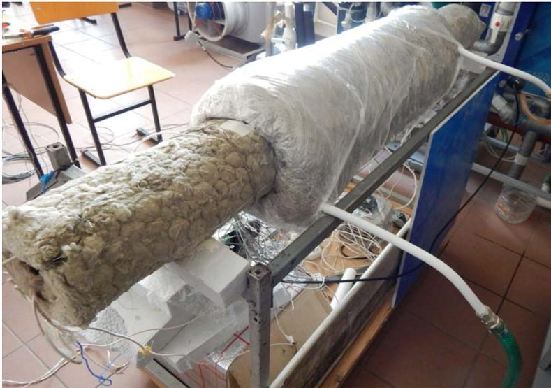
Fig. 4. Experimental investigation of thermal conductivity. Rock wool insulation wrap around hot pipe.
