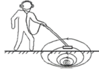
Fig .3. Induced signals in the induction method.
