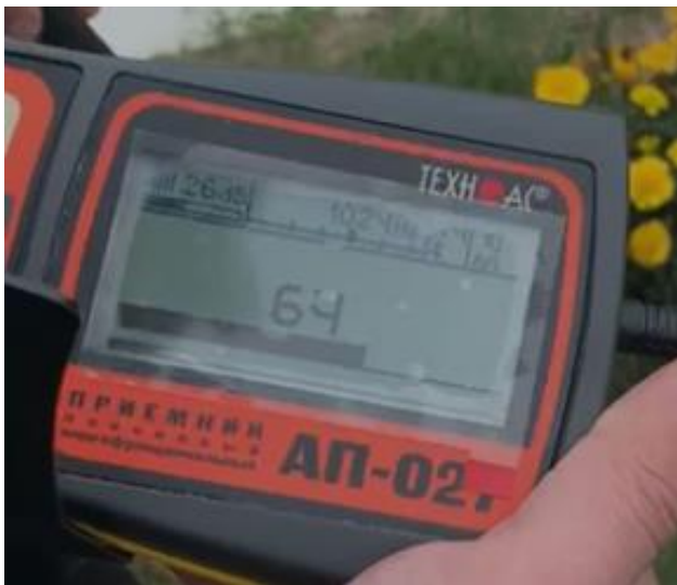
Fig .2. Line locator system receiver
