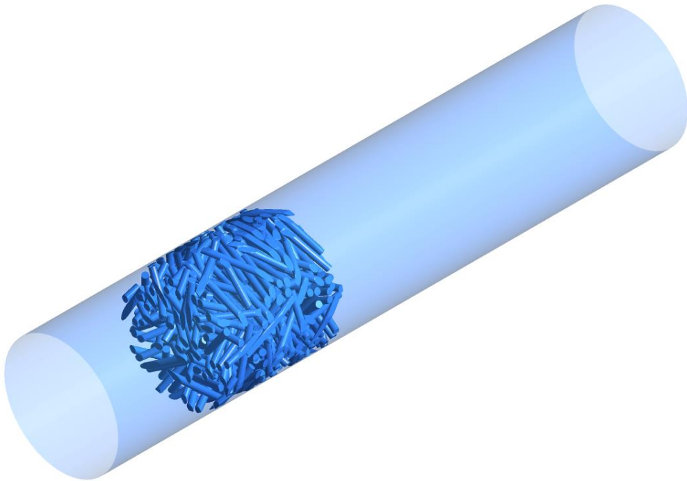
Fig. 1. An example of a calculation domain with fibrous material porosity \varepsilon = 0.7 .
