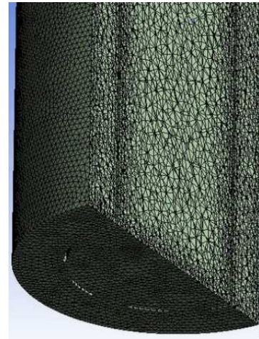
Fig. 2. Development of computational grid for a solid-state model of a multi-vortex contact device
