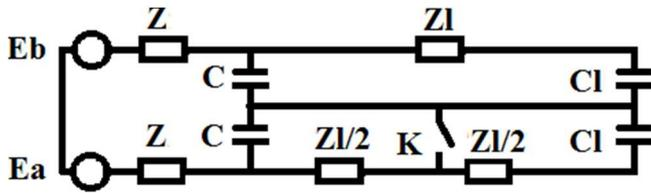
Fig. 2. Line model in SPEF mode without one unfault phase line
