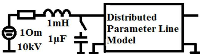
Fig. 6. Signal "Damped Oscillations" generation circuit
