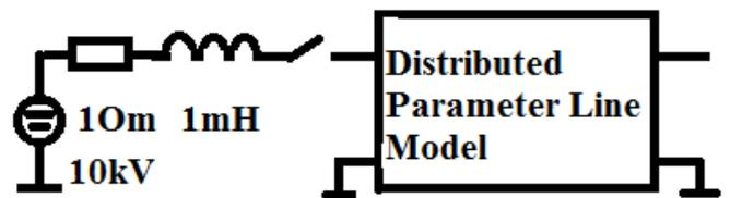
Fig. 4. Signal "Voltage step" generation circuit
