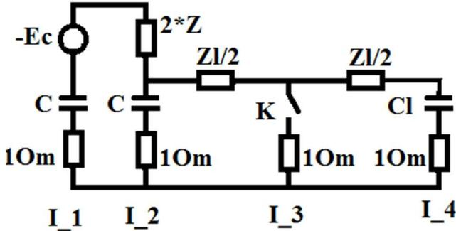
Fig. 3. The simplest three-contour line model in the SPEF mode
