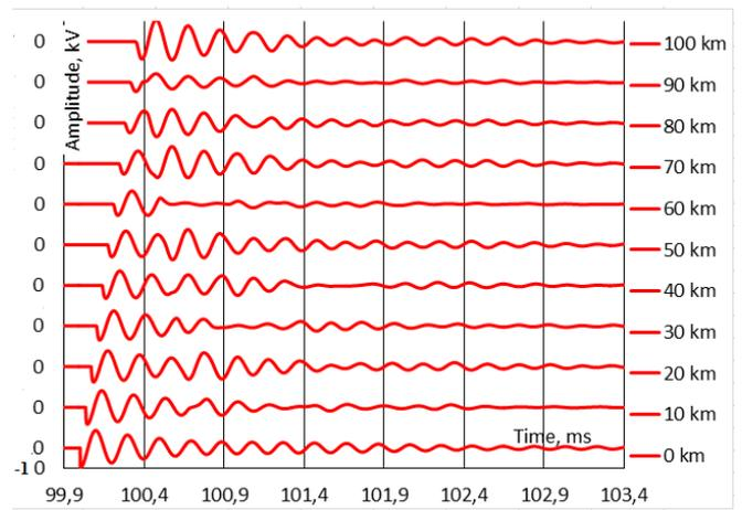
Fig. 7. Oscillograms of the resulting signals at different distances from the beginning of the line during the generation of "Damped Oscillations"
