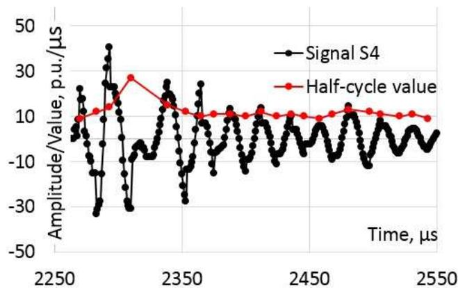
Fig. 12. Time dependence of the value of the half-period of oscillations
