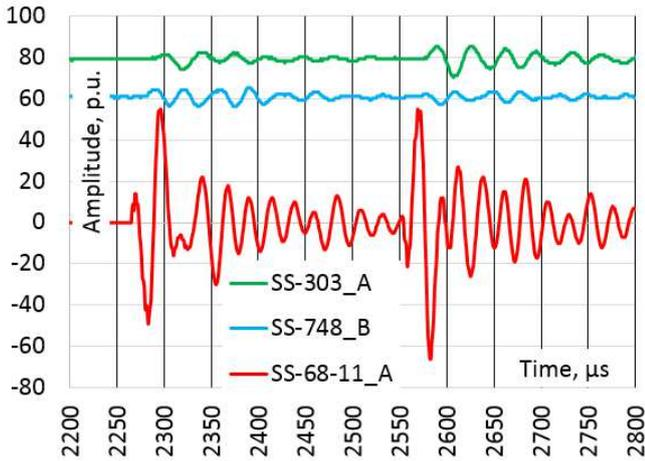
Fig. 9. Synchronous waveforms at different points in the network
