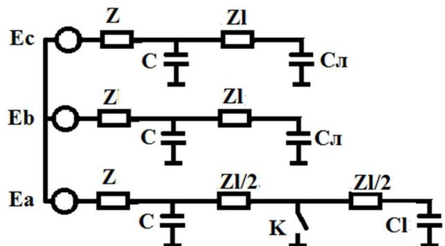
Fig. 1. Line model in SPEF mode
