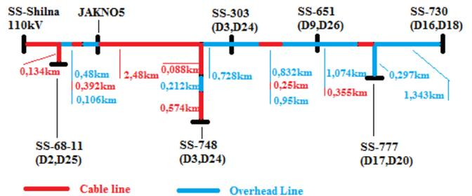
Fig. 8. Diagram of a tree-like electrical network
