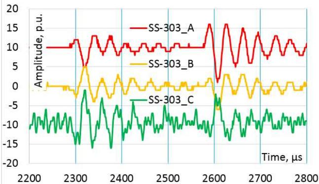
Fig. 10. Synchronous oscillograms in different phases of the line
