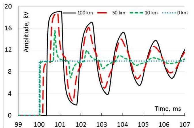
Fig. 5. Oscillograms of the resulting signals at different distances from the beginning of the line during the generation of "Voltage step"
