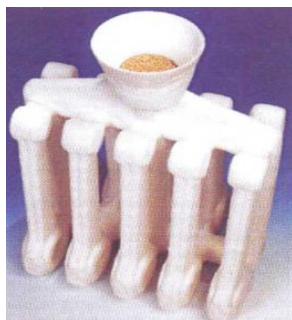
Figure 1 - Ceramic mold with foam ceramic filter installed
