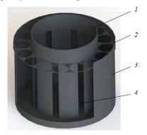
**Fig. 1.** A three-dimensional model of centrifugal separation device with coaxially arranged pipes (cross-section view): 1 - inlet nozzle of inner cylindrical pipe, 2 - grid with round holes, 3 - body of separation device, 4 - rectangular holes.
