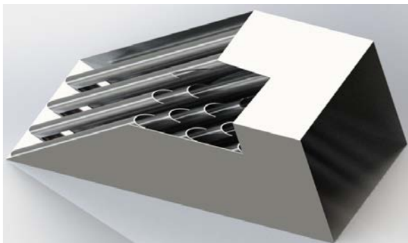
Fig. 1. 3D model of a rectangular separator (section view).
