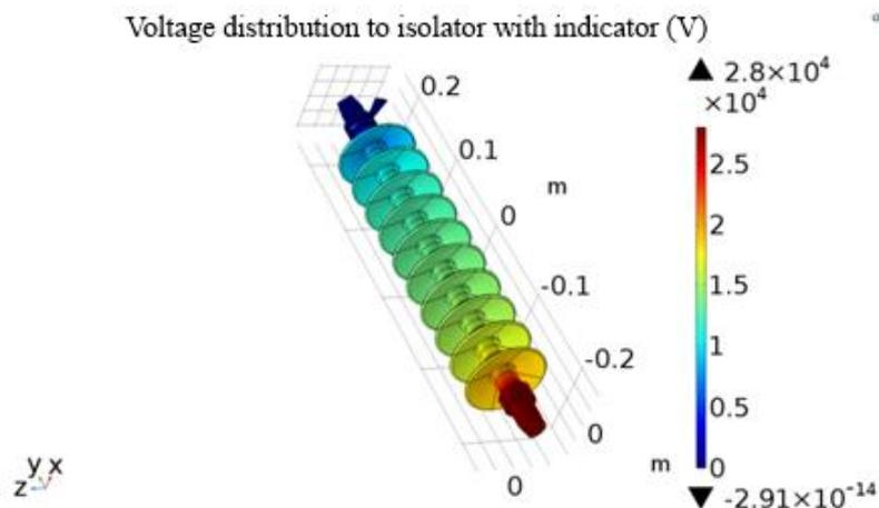
**Figure 6.** Voltage distribution on insulator in color.
