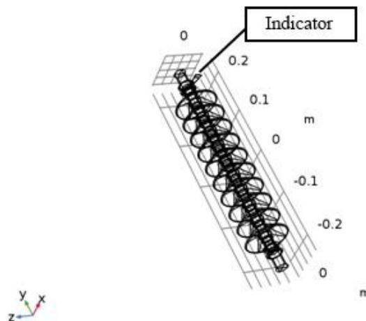
**Figure 3.** Geometry of three-dimensional model of LK 70/35 insulator with indicator installed at the upper end.
