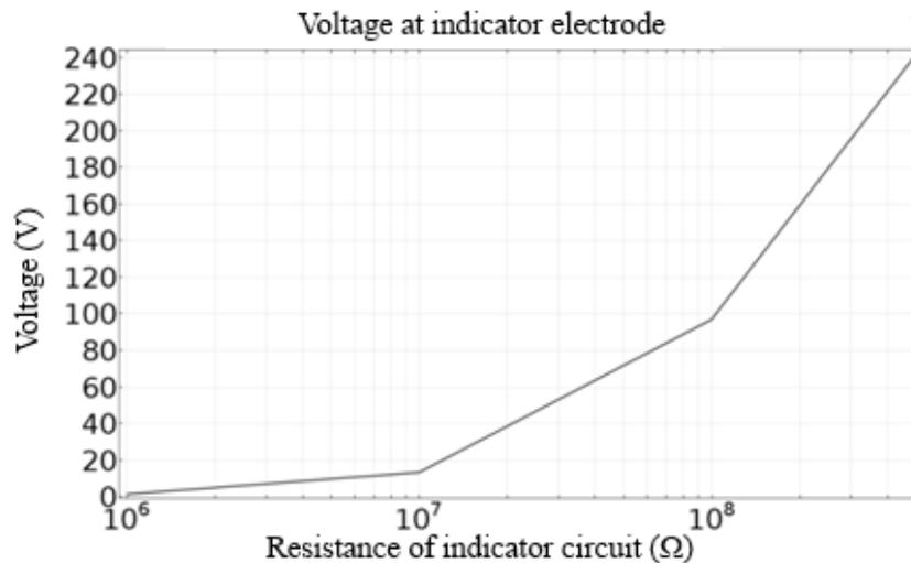
**Figure 8.** Dependence of amplitude value of circuit voltage on resistance of indicator circuit.
