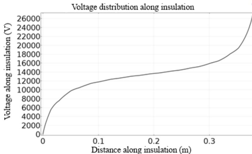
**Figure 7.** Voltage rise plot at insulator from grounded end to energized end.
