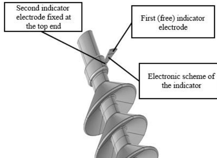
**Figure 4.** Indicator attached to the top end.
