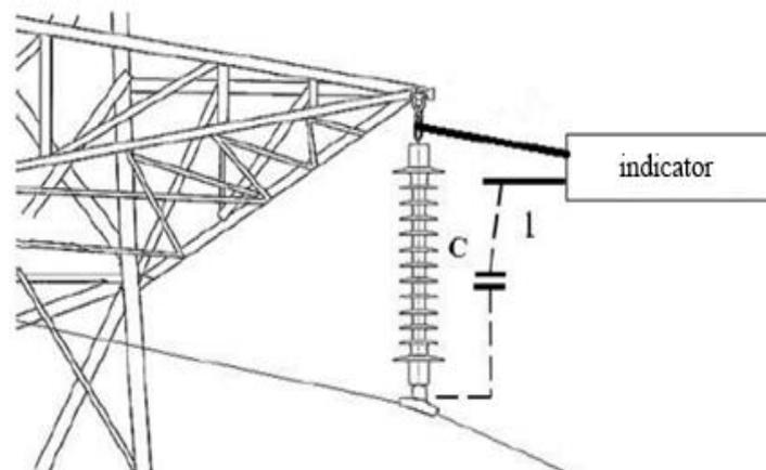
**Figure 1.** Indicator in the electric field near the insulator.
