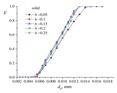
Figure 2. The efficiency of particle deposition on a single solid fiber for various h.
