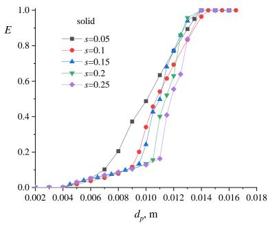
**Figure 4.** The efficiency of particle deposition on a single solid fiber for various *s*.
