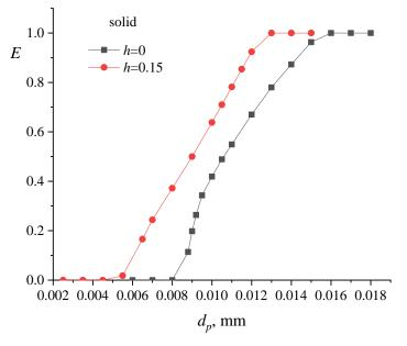
**Figure 3.** The efficiency of particle deposition on a single solid fiber for h without a protrusion and with a protrusion of 0.15 mm.
