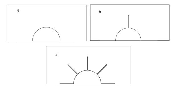
**Figure 1.** The scheme of the protrusion location on the filter fiber: 0 - fiber without protrusion, h - fiber with one protrusion, s - fiber with five protrusions.
