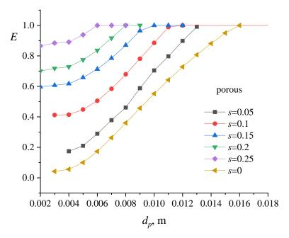
**Figure 7.** The efficiency of particle deposition on a single porous fiber for various *s*.
