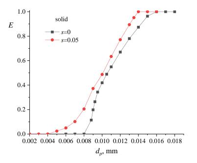
**Figure 5.** The efficiency of particle deposition on a single solid fiber for two various s – without a protrusion and with a protrusion of 0.05 mm.
