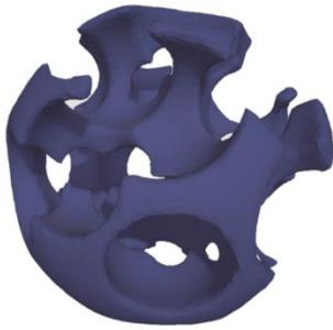
**Figure 1.** Model of a granule with the porosity  $\varepsilon = 0,8$ .
