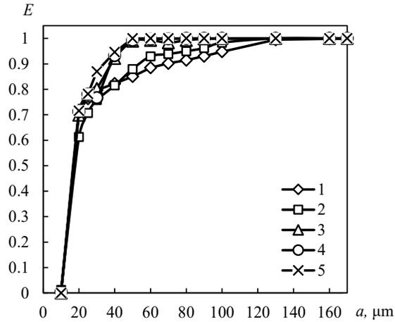
**Fig. 4.** Efficiency of straight arc-shaped separation device  $E$  against particle diameter  $a$  at different number of rows of arc-shaped elements  $N$ : 1 – 4; 2 – 6; 3 – 8; 4 – 10; 5 – 12. Basic parameters:  $h = 250$  mm,  $W = 1$  m/s,  $\rho_a = 3400$  kg/m<sup>3</sup>.
