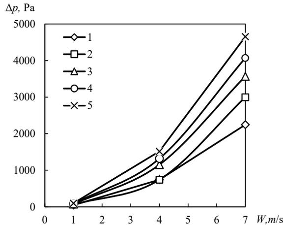
**Fig. 6.** Pressure drop of separation device  $\Delta p$  against gas inlet velocity  $W$  at different number of rows of arc-shaped elements  $N$ : 1 – 4; 2 – 6; 3 – 8; 4 – 10; 5 – 12.
