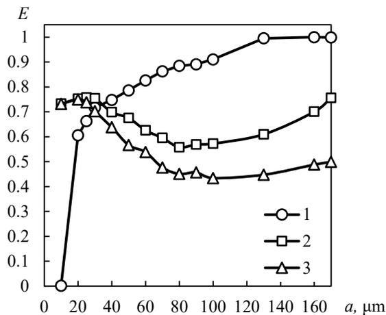
**Fig. 3.** Efficiency of the straight arc-shaped separation device  $E$  against particle diameter  $a$  at different inlet gas inlet velocities  $W$ , m/s: 1 – 1; 2 – 4; 3 – 7. Basic parameters:  $h = 250$  mm,  $N = 4$ ,  $\rho_a = 3400$  kg/m<sup>3</sup>.
