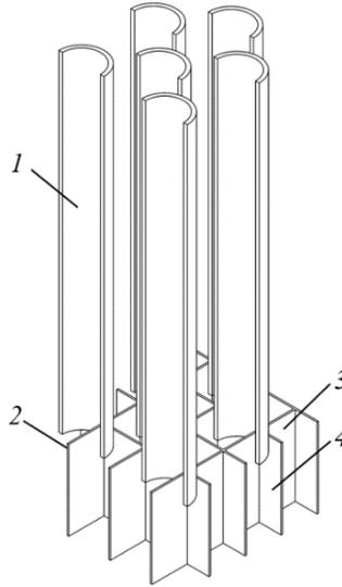
**Fig. 2.** Diagram of the main unit of the separation device: 1 – arc-shaped elements; 2 – screen; 3 – longitudinal plates; 4 – transverse plates.
