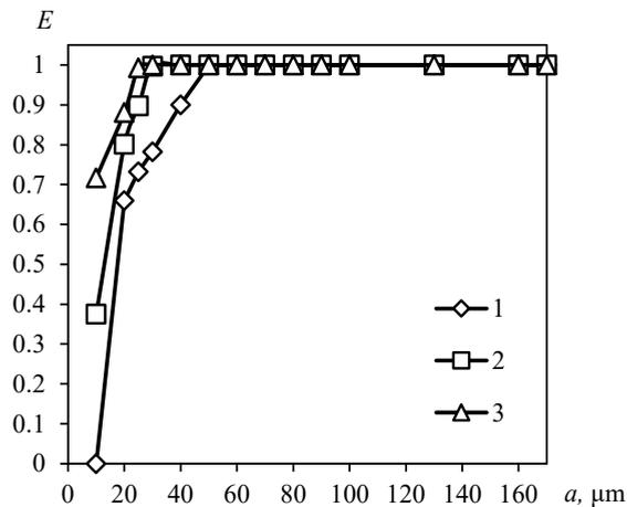
**Fig. 5.** Efficiency of straight arc-shaped separation device  $E$  against at different density  $\rho_a$ , kg/m<sup>3</sup>: 1 – 3400; 2 – 7000; 3 – 10000. Basic parameters:  $h = 250$  mm,  $W = 1$  m/s,  $N = 12$ .
