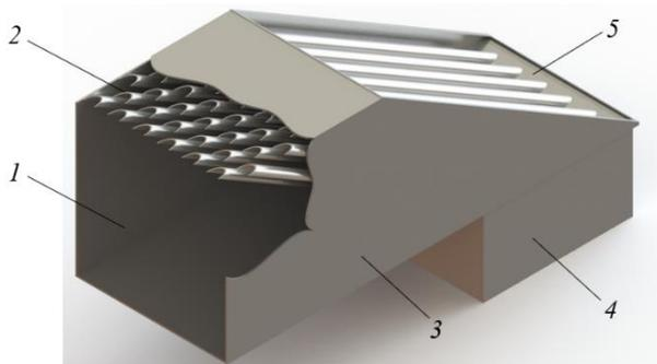
**Fig. 1.** 3D model of the separation device with arc-shaped elements: 1 – dusty gas inlet; 2 – arc-shaped element rows; 3 – body; 4 – bunker; 5 – gas outlet.
