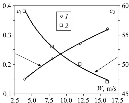
**Fig. 6.** Dependences of the coefficients of the sigmoid function  $c_1$  (1) and  $c_2$  (2) on the inlet velocity of the gas flow in the multi-vortex classifier–separator.
