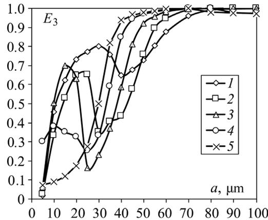
**Fig. 5.** Dependences of the efficiency of three multi-vortex classifiers–separators with coaxially located pipes on the particle size of silica gel (inner pipe with a conical transition) at the inlet gas flow velocity  $W$ : 1 – 2 m/s; 2 – 4 m/s; 3 – 8 m/s; 4 – 12 m/s; 5 – 16 m/s.
