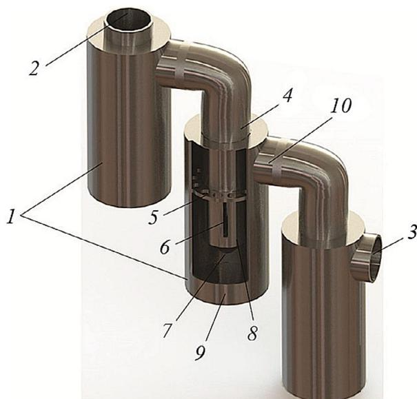
**Fig. 1.** 3D model of three series-connected classifier–separators with coaxial pipes: 1 — multi-vortex classifiers–separators; 2 — inlet pipe to the group of devices; 3 — outlet pipe from the group of devices; 4 — inlet part of the pipe to the apparatus 2; 5 — plate with round holes; 6 — rectangular slots; 7 — hole with a conical transition; 8 — inner pipe; 9 — outer pipe; 10 — outlet part of the pipe from the apparatus 2.
