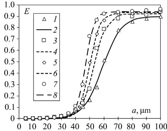
**Fig. 4.** Dependences of the efficiency of one multi-vortex classifier–separator with coaxially located pipes on the particle size of silica gel (inner pipe without a conical transition) at gas velocity  $W$ : 1, 2 — 4 m/s; 3, 4 — 8 m/s; 5, 6 — 12 m/s; 7, 8 — 16 m/s; icons — calculated values of  $E$ ; lines are sigmoid functions indicating the change in efficiency at the corresponding flow rate.
