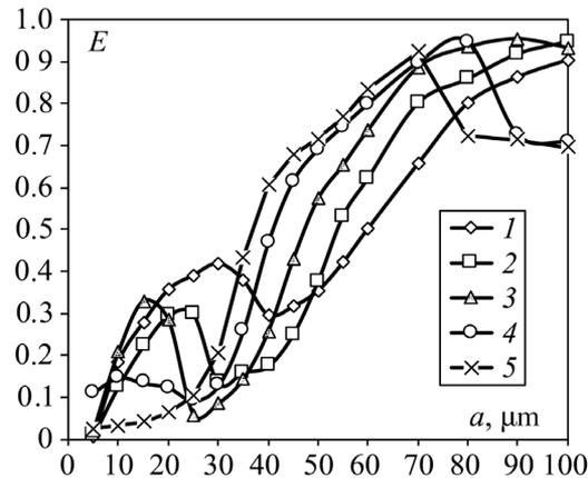
**Fig. 3.** Dependences of the efficiency of one multi-vortex classifier–separator with coaxially located pipes on the particle size of silica gel (inner pipe with a conical transition) at the inlet gas flow velocity  $W$ : 1 – 2 m/s; 2 – 4 m/s; 3 – 8 m/s; 4 – 12 m/s; 5 – 16 m/s.
