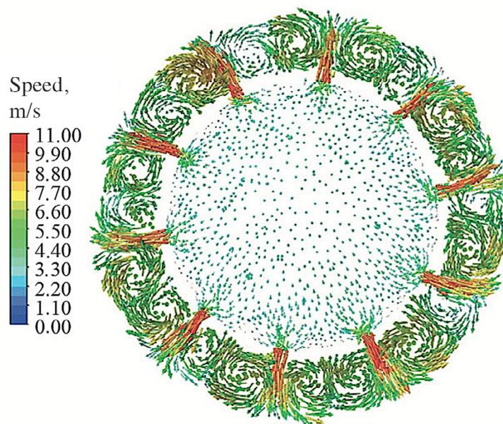
**Fig. 2.** Diagram of gas swirls in the annulus of a multi-vortex classifier–separator (top view), obtained by modeling in Ansys Fluent.
