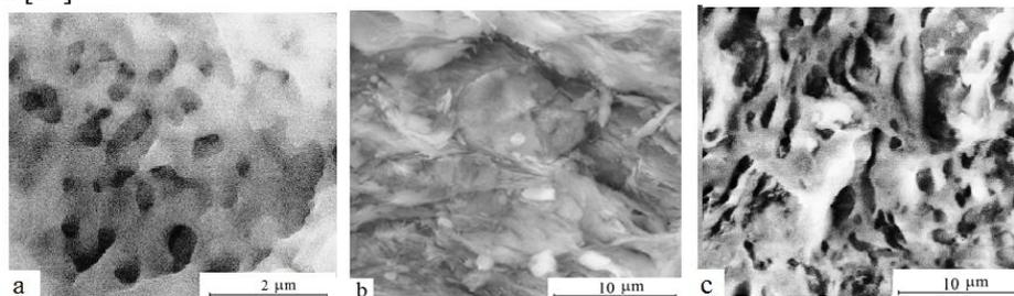
**Fig.1.** Microstructure of compositions sintered in the microwave field of compositions: a - silica fume + NaCl, b - marl + silica fume, c - marl + silica fume + NaCl.
