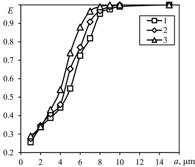
**Figure 4.** Separation efficiency versus particle size under different particle densities  $\rho_a$ ,  $\text{kg/m}^3$ : 1 – 2000; 2 – 2330; 3 – 3000. Inlet gas velocity  $W = 7$  m/s.
