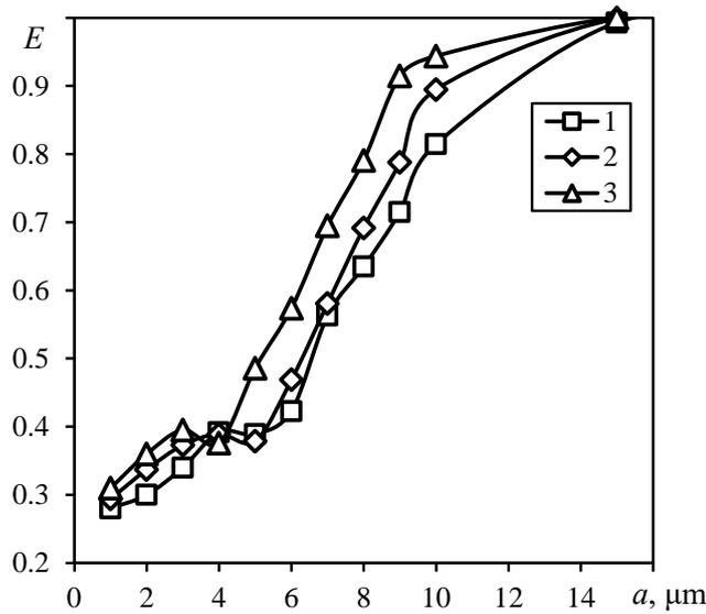
**Figure 2.** Separation efficiency versus particle size under different particle densities  $\rho_a$ ,  $\text{kg/m}^3$ : 1 – 2000; 2 – 2330; 3 – 3000. Inlet gas velocity  $W = 3$  m/s.
