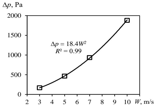
**Figure 6.** Pressure loss versus inlet gas velocity.
