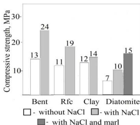
**Figure2.** Durability on compression of the samples burned at 1000°C from: bentonite clay – Bent, refractory clay - Rfc, clay - Clay, Diatomite.
