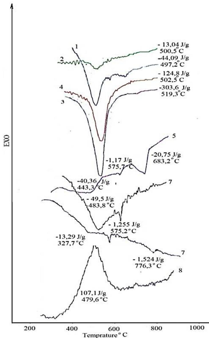
**Figure 1.** Thermograms (DTA): 1 – bentonite clay, 2 – bentonite clay and NaCl, 3 – refractory clay, 4 – refractory clay and NaCl, 5 – clay and NaCl, 6 – diatomite with NaCl and marl, 7 diatomites with NaCl, 8 – diatomite.
