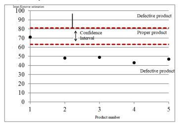
Fig 10. The principle of decisive "proper - defective" rule development by the example of Iman-Konover estimate
