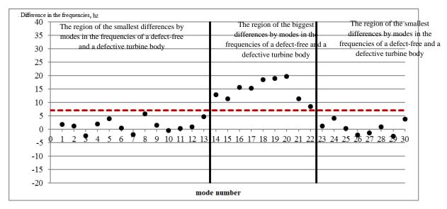
Fig 5. Difference in the frequencies of a defect-free and a defective TC turbine body from the mode 1 to 30
