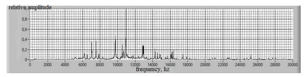
Fig 12. The reference spectrum of TC turbine bodies
