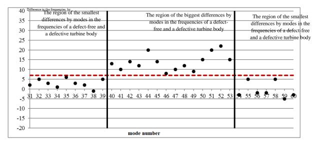
Fig 6. Difference in the frequencies of a defect-free and a defective TC turbine body from the mode 31 to 60
