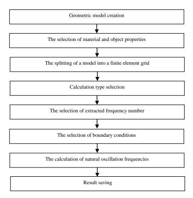
Fig 3. Calculation flowchart
