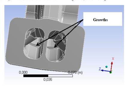
Fig 2. Defective body of TC turbine
