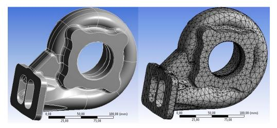
Fig 1. Three-dimensional model (on the left) and a finite-element grid (on the right) of TC turbine body
