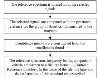
Fig. 4. Sequence of work of the subprogram "Formation of reference spectra".
