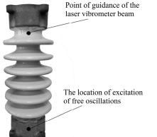
Fig. 6. Point of guidance of the laser vibrometer beam and the location of excitation of free oscillations
