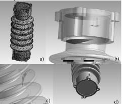
Fig.1. a – finite-element model of the SRI, b – crack of the insulator's trunk, c – crack of the insulator rib, d – hard seal.
