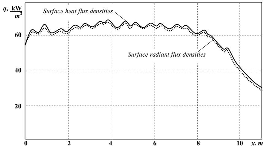
Figure 4. Distribution of surface densities of heat fluxes along the height of the tubular screen.
