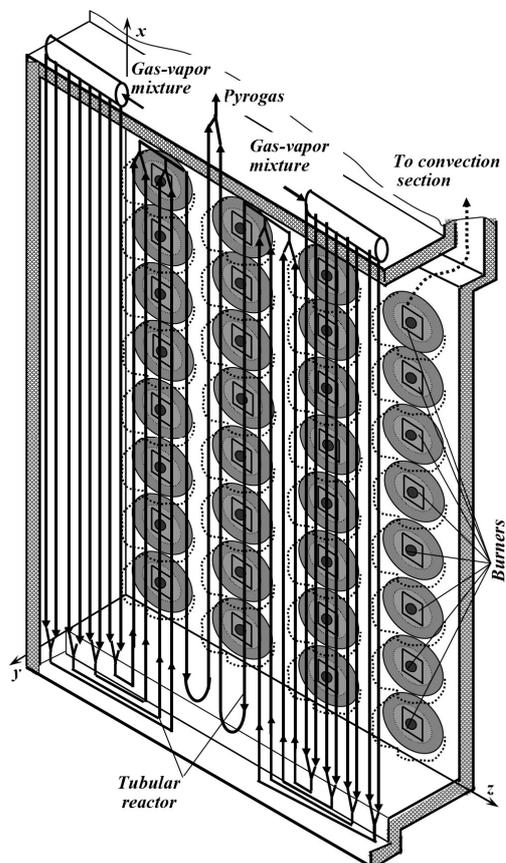
Figure 1. Scheme of the fourth part of radiation chambers of a tubular furnace ethane pyrolysis and coordinate system.
