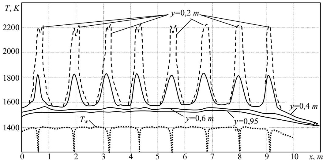
Figure 3. Changes in the temperature of the combustion products at different distances from the side wall ( $y$ ) and the inner surface of the lining ( $T_w$ ) along the height of the furnace.
