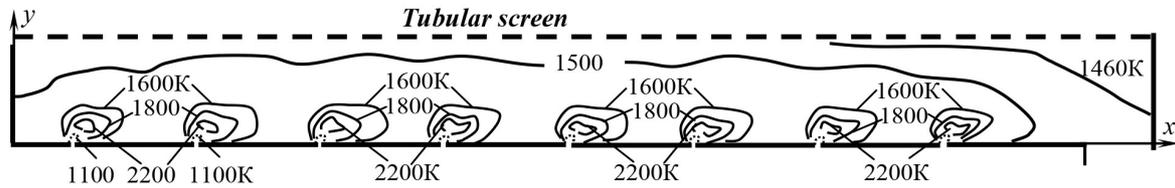
Figure 2. View of isotherms in the radiation chamber of a tubular ethane pyrolysis furnace
